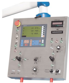
Equipped with electronic hand-wheels and extended milling functions the Servomill offers the advantages of modern CNC technology in conventional machining
