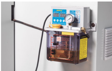
Continuous precision lubrication minimizes friction and wear of movable parts and increases the machine life
